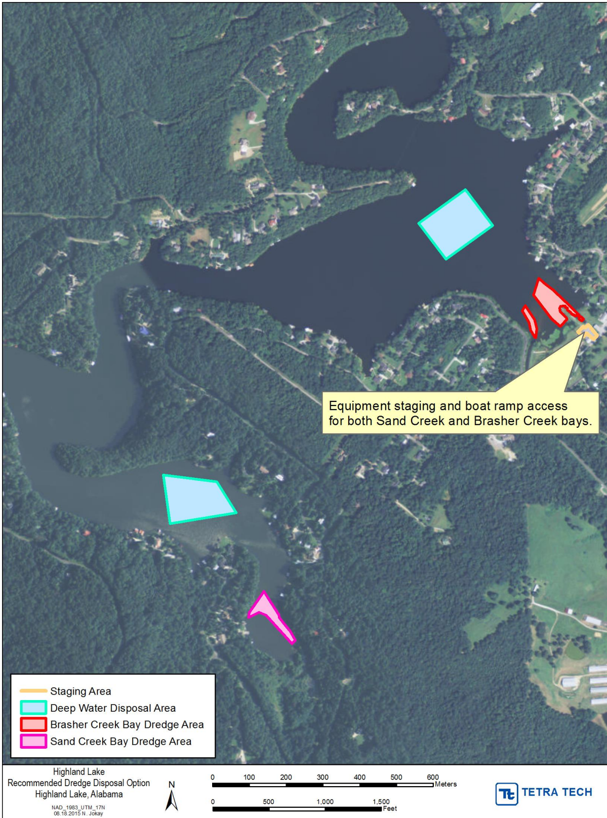
Figure 13. Recommended dredging and disposal plan overview
